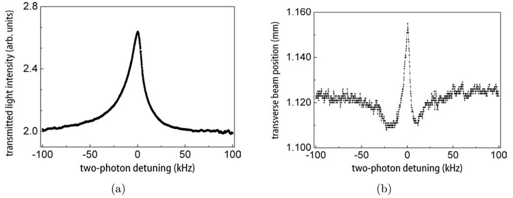
**Figure 4.** (a) Signal beam transmission spectrum. The two-photon detuning is given by  $\delta = \omega_S - \omega_C + \mu_B \cdot B$ , with the optical frequencies of the signal and the control beam,  $\omega_S$  and  $\omega_C$ , the Bohr magneton  $\mu_B$  and the magnetic bias field  $B$ . (b) Signal beam position transverse to the optical axis. For a two-photon detuning near zero, a clear deflection of the signal beam is observed.
