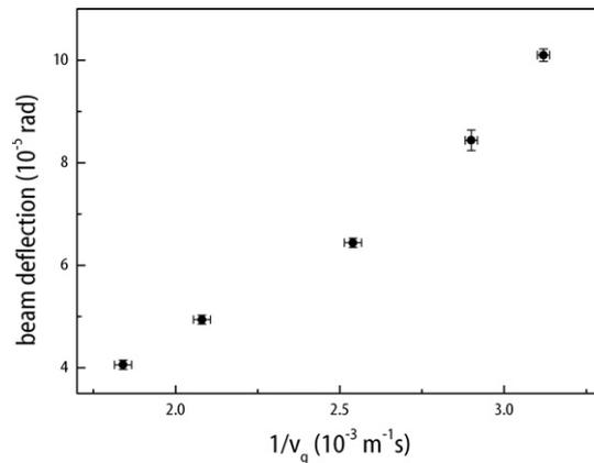
**Figure 5.** Dependence of the deflection of the signal beam on two-photon resonance on the inverse group velocity.
