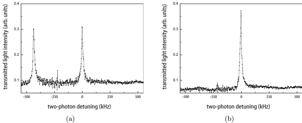
**Figure 7.** Signal beam transmission spectra. Each spectrum is the average of ten measurements. (a) The magnetic field is oriented transversely to the optical beam axis (see figure 6). The signal and control beams are linearly polarized, where the polarization of the control beam is aligned collinear to the magnetic field. (b) Corresponding spectrum for a longitudinal magnetic field configuration and opposite circular polarizations of the optical beams, as has been shown in figure 1.
