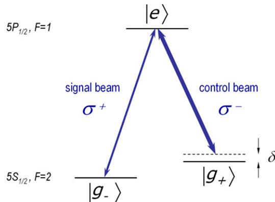
**Figure 1.** Simplified diagram of the  $\Lambda$ -type three-level system relevant to the experiments with longitudinal magnetic bias fields. Two ground states,  $|g_{-}\rangle$  and  $|g_{+}\rangle$ , are coupled to the spontaneously decaying excited state  $|e\rangle$  via a  $\sigma^{+}$ -polarized signal beam and a  $\sigma^{-}$ -polarized control beam.  $\delta$  denotes the two-photon detuning.
