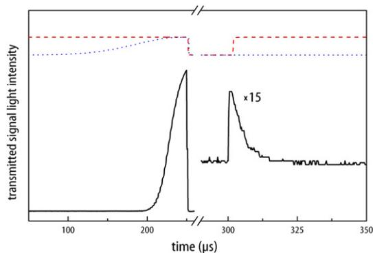
**Figure 8.** Stored light measurement carried out in the transverse magnetic field configuration. The signal background due to residual control beam transmission has been subtracted from this plot. The transmitted signal beam intensity is averaged and the signal of the retrieved pulse is magnified by a factor of 15. Above the data, the representations of signal (dotted line) and control (dashed line) beam intensities are shown.
