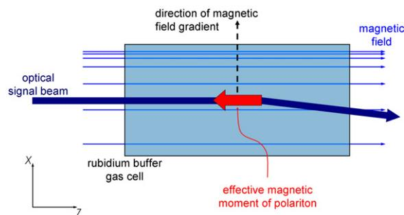
**Figure 3.** Schematical representation of a Stern–Gerlach experiment for slow light based on a magnetic bias field longitudinal to the beam propagation axis. The transverse magnetic field gradient causes a deflection of the signal beam, which is attributed to the dark polariton possessing an effective magnetic moment.
