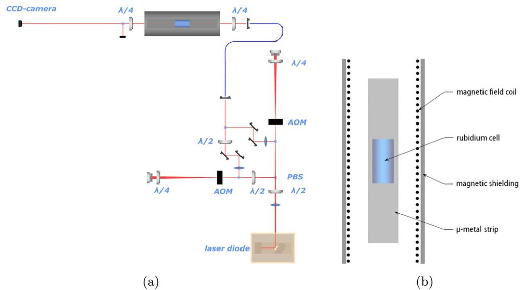
**Figure 2.** (a) The optical set-up. (b) Detailed view of the rubidium cell apparatus.
