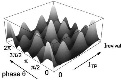
FIG. 3. Calculated interference signal for an  $F=4$  to  $F'=4$  transition as function of both the phase of the second Ramsey pulse  $\theta$  and the tensor polarizing beam intensity  $I_{TP}$ . The vertical scale gives the ratio  $|\langle \varphi_d(T) | \varphi_d(0) \rangle|^2$  of atoms in the dark state after the pulses to those initially in that state.
