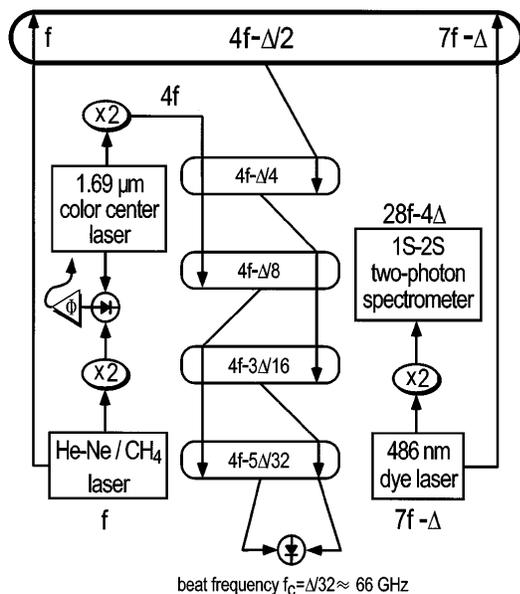
FIG. 2. Experimental setup for the comparison of the 1S-2S two-photon resonance at 243 nm with a  $3.39 \mu\text{m}$  methane-stabilized He-Ne laser. The large-gap divider on top finds the midpoint between  $f$  and  $7f - \Delta$ :  $4f - \Delta/2$ . The difference to  $4f$  is then further reduced using the cascaded divider stages.
